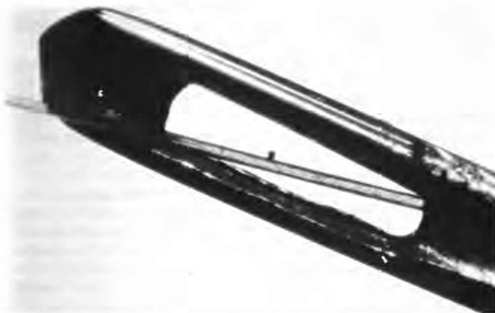
Fig. 30. A tiny laser fusion fuel pellet suspended on a human hair in the eye of a needle. (Courtesy of the United States Department of Energy.)
