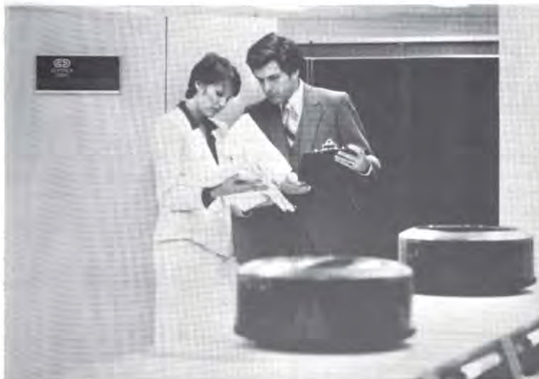
FIGURE 4.34. The CDC CYBER 205 can perform up to 800 million operations per second and has four million words of central memory. (Courtesy Control Data Corporation)
