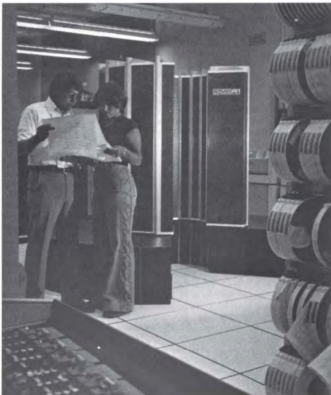
FIGURE 4.33. The Cray-1S supercomputer is a cylindrical circuit array to minimize the length of electrical connections. (Courtesy Los Alamos Scientific Laboratory)
