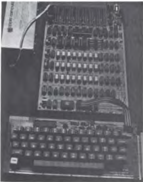
FIGURE 4.24. The main circuit board of the Apple-II computer showing the principal components of a digital computer. (Courtesy Apple Computer, Inc.)
