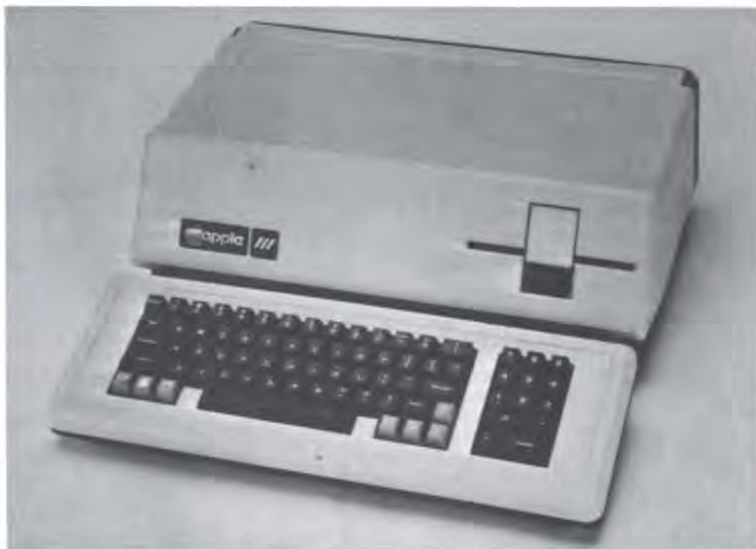
FIGURE 4.15. The keyboard of the Apple-III computer provides an example of the ASCII format. (Courtesy Apple Computer, Inc.)
