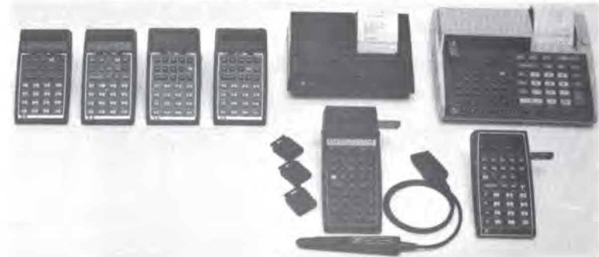
FIGURE 4.32. The evolution in hand-held calculators from simple four-function units (+, −, ÷, ×) to microprocessor-based units approaching a personal computer in capability has been quite rapid. (Courtesy Hewlett-Packard Company)
