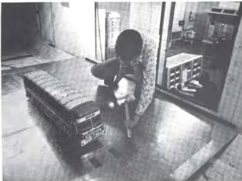
FIGURE 2.20. Windtunnel testing of a bus model. (Courtesy University of Michigan College of Engineering)
