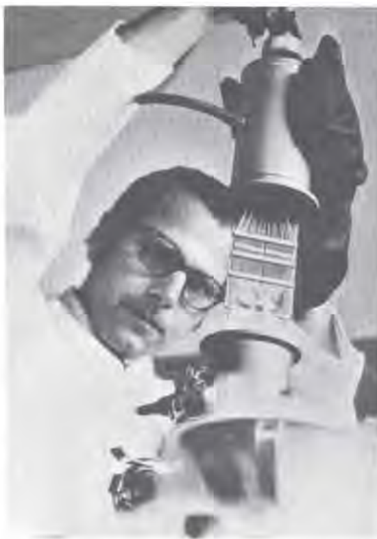
FIGURE 4.35. The experimental Josephson circuit computer will operate at supercooled temperatures at speeds orders of magnitude faster than semiconductor-based computers. (Courtesy IBM Corporation)
